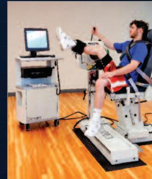
Objective testing provides valuable, isolated muscle-performance data for pre-emptive injury screening, managing rehabilitation and determining readiness for return to play.
