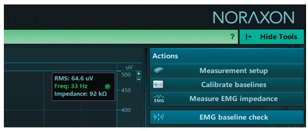
Built-in impedance checker and signal quality monitor
